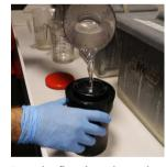
Pour the fixer into the tank. Agitate first 30 sec and then 10 sec every half minute.
