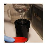
Pour the stop bath into the tank. Agitate continuously by gently swirling and inverting the tank.
