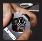
Open a film cassette. Use the rounded end of the bottle cap opener to pry off the flat end of the cassette.
