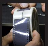
Push the film about 5cm into the reel. Wind the film into the reel by turning the two halves of the reel forwards and backwards.
