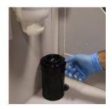
Fill the tank with water. Invert the tank 5 times. Drain it away and refill. Invert the tank 10 times. Once more, drain the water. Invert the tank 20 times and drain it away. Repeat the last step three times.
