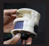
Cut the spool free when all the film is wound. Put the reel in the tank and cover it.
