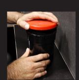
When the loaded reel is in the tank with the cover securley in place you can trun on the lights.
