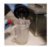
When developing time is up, pour out the developer.
