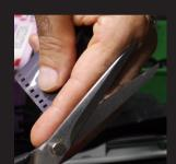
Cut off the tongue to make the end of the film square. Also cut off the corners. Hold the film loosely by its edges.
