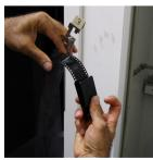
Attach clothes pin to the beginning and end of film as a bottom weight. Hang the film on the dryer. Press both buttons on the dryer and set to 40 min.
