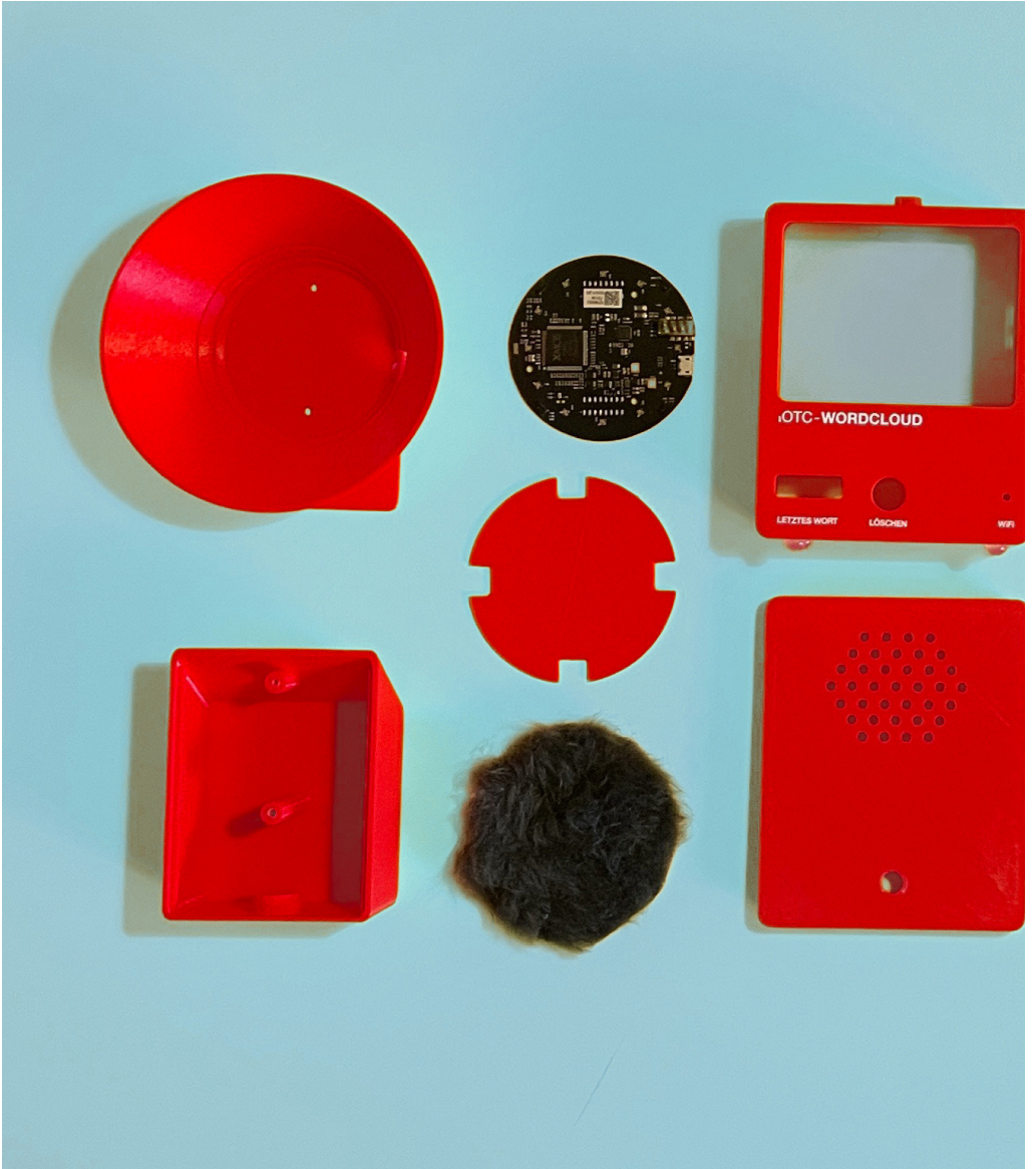
All components of the WordCloud laid out and ready to be assembled
