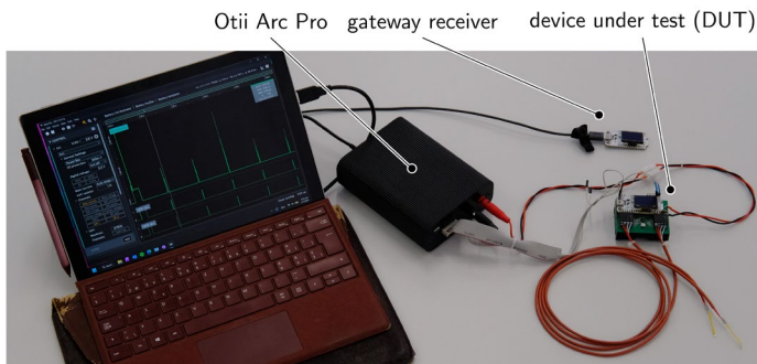
Current consumption of the data logger (DUT) was measured using the Otii Arc Pro power profiler. A dedicated ESP32-S3 was used as the receiver for ESP-NOW transmissions.
