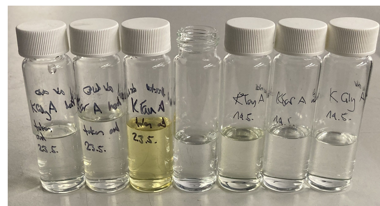
Fig 2: Solvent samples after CO 2 absorption: thermally cycled >200 times left, <10 times right
