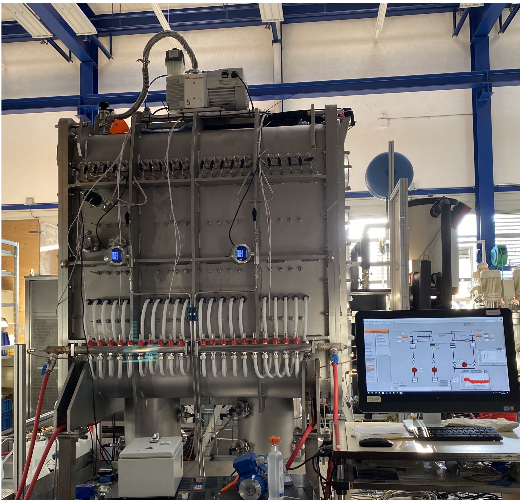
Sorption heat storage demonstrator
