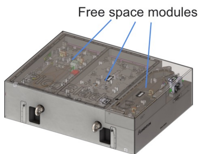
Figure 1. Ultrafast lasers free space modules containing optical components
