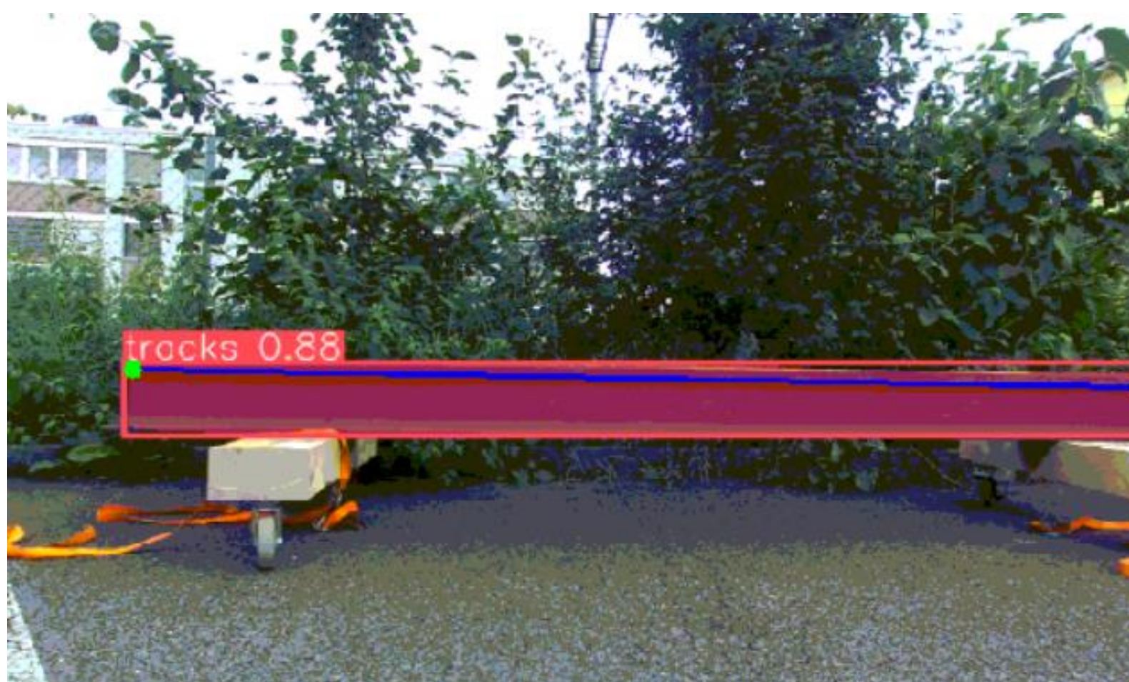
Fig.4 Track Detection and Hough Line Extraction
