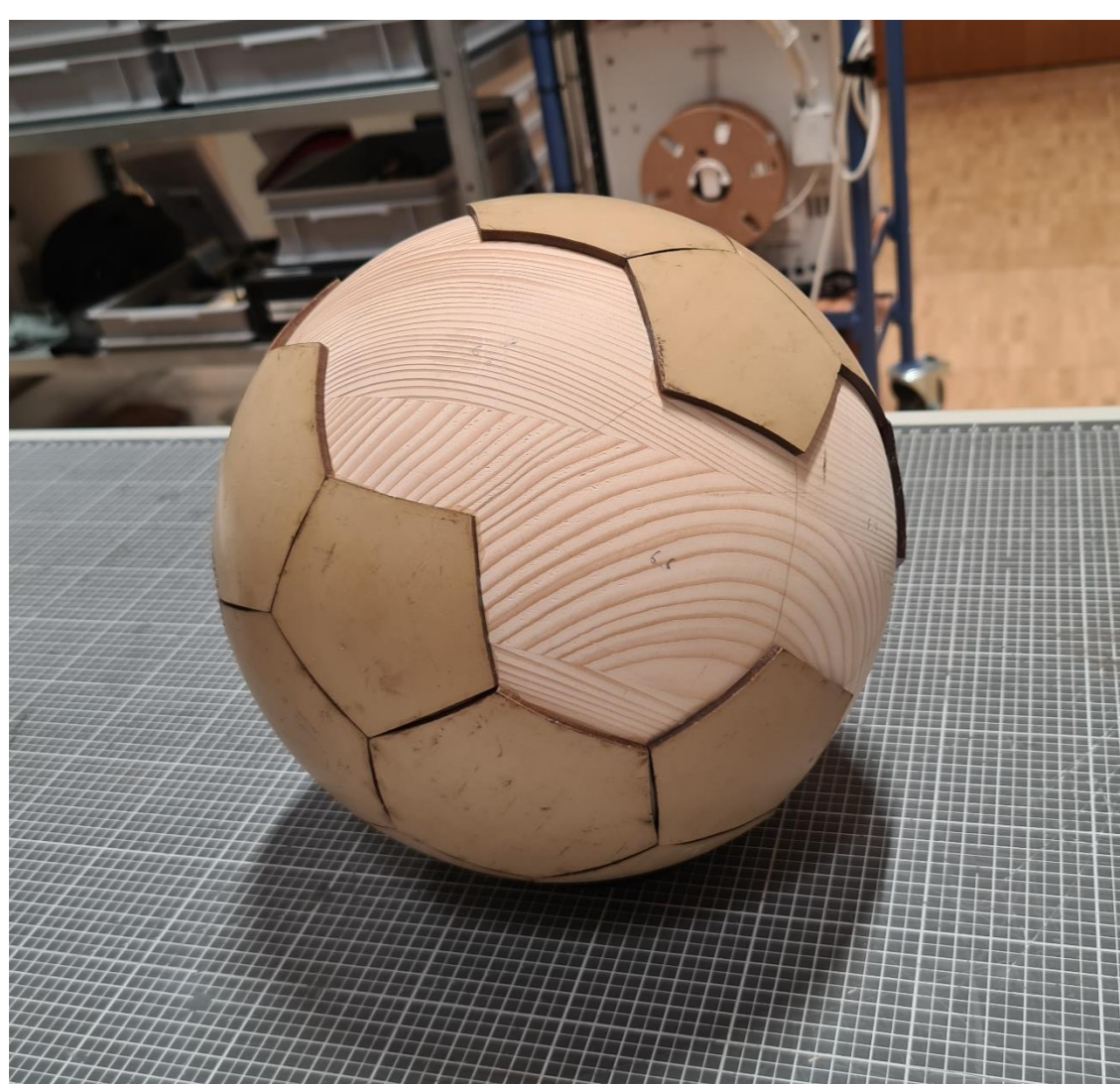
Ball made of a wooden core coated with rubber tiles
