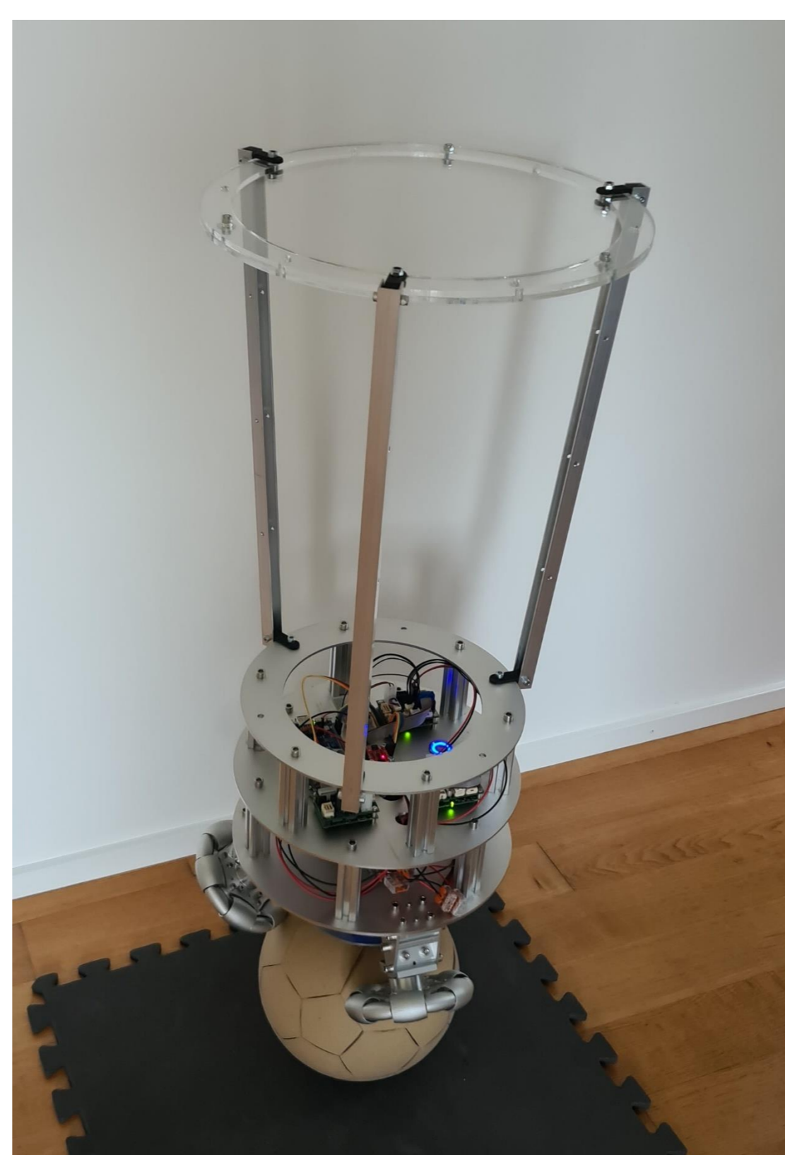
Ballbot balancing with platform
