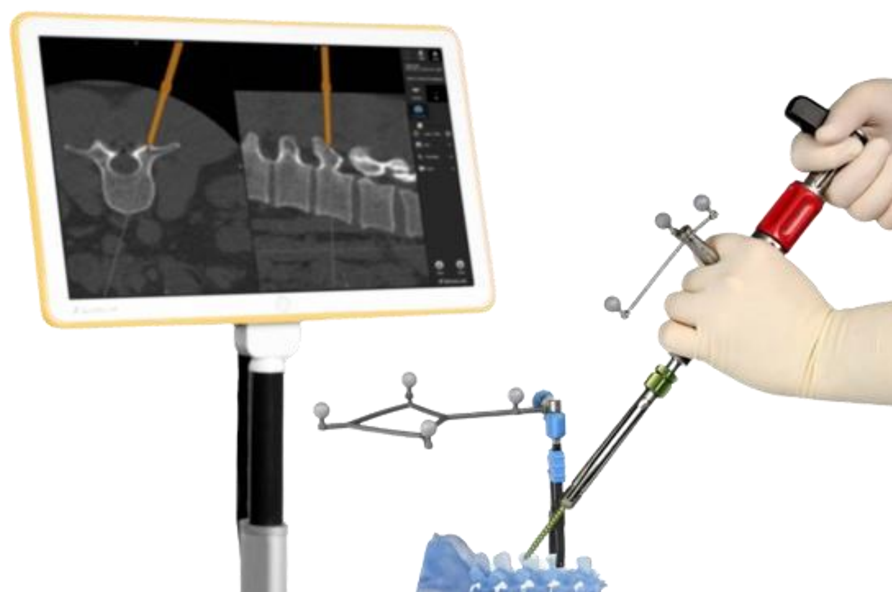
Intraoperative navigation systems allow the spine and the surgical instruments to be displayed on a navigation screen. (Source: BrainLab)
