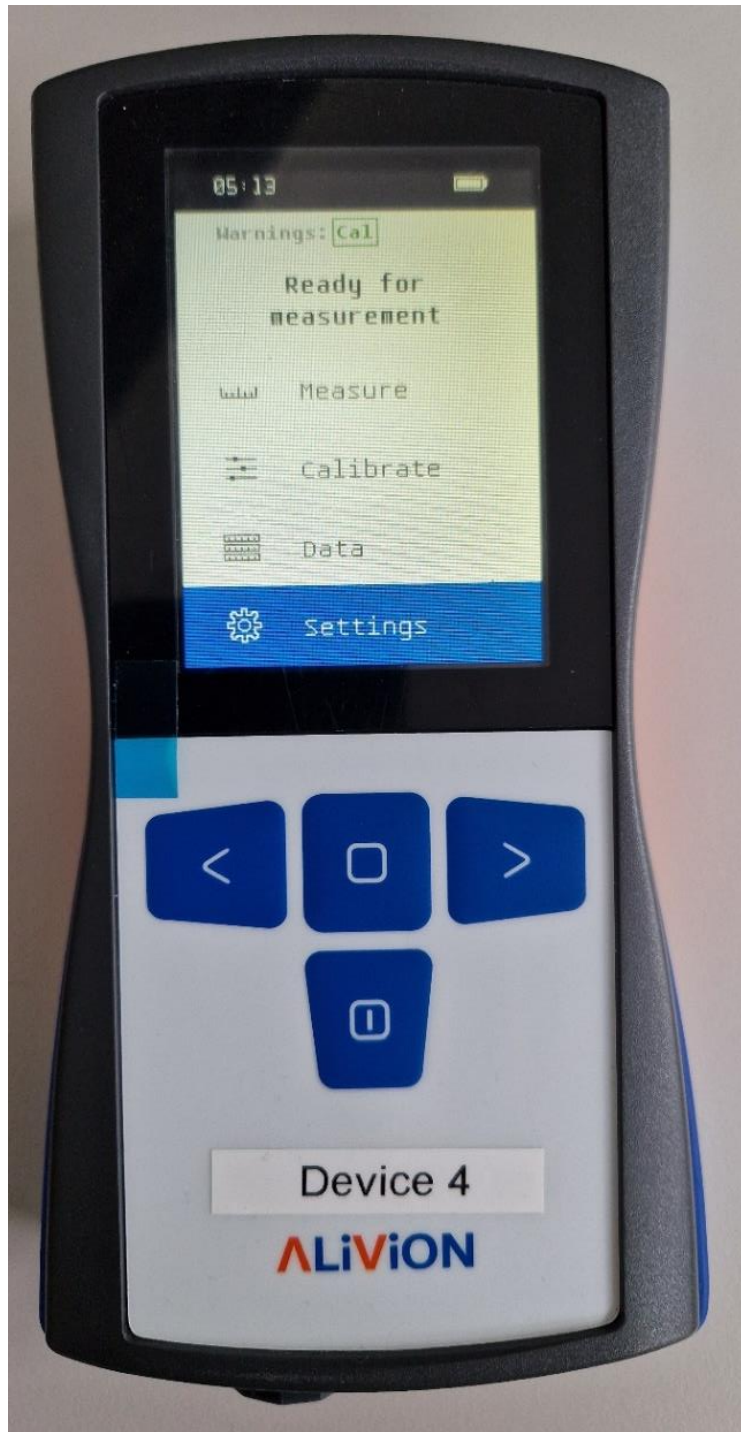
Figure 1: Breath Acetone Detector from Alivion AG, used for non-invasive measurement of acetone levels.
