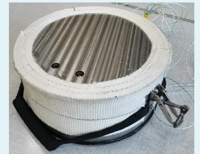
Figure 2: Functional model using PCM as latent storage (Estermann, 2023)
