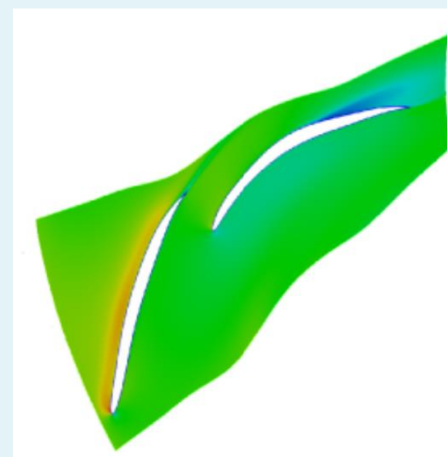
Figure 5: CFD results after performing an Adjoint optimization
