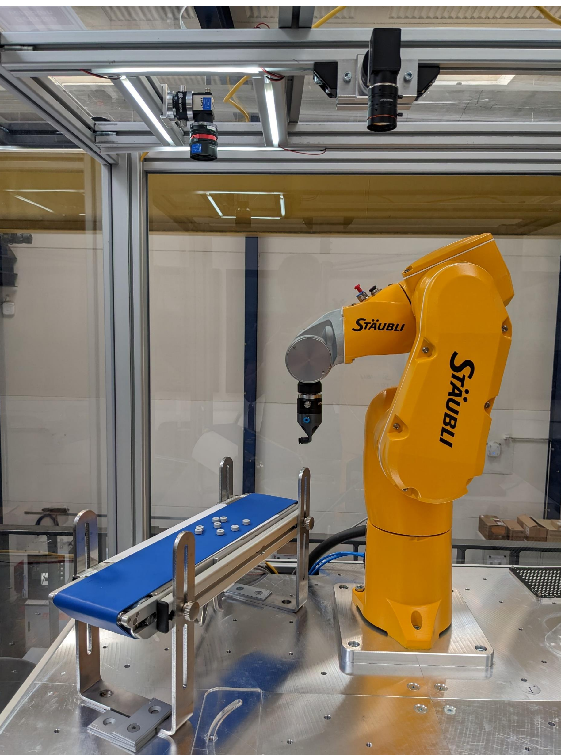
Fig. 2: The test setup with the monocular camera and top illumination (top of the image), the parts on the blue conveyor belt and Stäubli robot.
