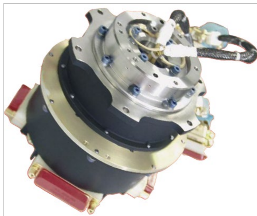
Figure 2: SEPTA 41; Solar Array Drive Mechanism [Source: oerlikon.com]
