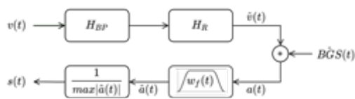
Abb. 1 The general structure of the auralization procedure: A voice signal v(t) passes through the bandpass filter ( H_{BP} ) and room filter ( H_R ) before BGS is added. Afterward, a fade-in and -out window ( w_f(t) ) is applied and finally, the signal \hat{a}(t) is scaled to \pm 1 leading to the output signal s(t) .
