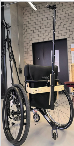
Figure 1: Measurement set-up Shows the with sensors, pressure mat and GoPro equipped wheelchair.
