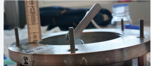
Figure 4: Side view on the ex-vivo model and emk-model. It shows the moving range of the emk-model. The mechanical model leg moves with the angle of the gears.
