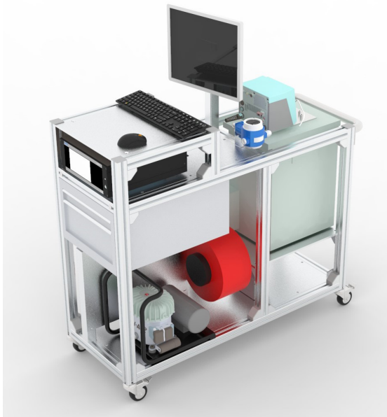
Fig. 1: Rendering of the mobile pressure and temperature sensor calibration module (PTCM)
