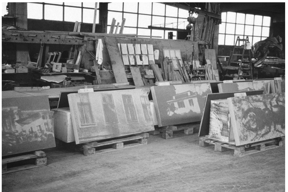
Abb. 36. Production process of imprinting on concrete panels. Preparation of elements.
