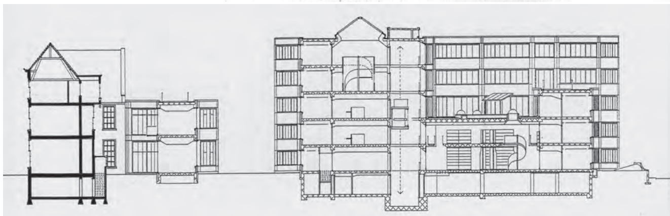
Fig. 29. Section showing Old mansion on left, new part with extended levels of old in the middle and new part with regular levels on right.
